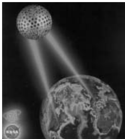
Fig. 23: Satellite laser ranging [LAGEOS LAsErGEOdynamics Satellite] by means of Nd:YAG pulse laser converting infrared wave length to green
