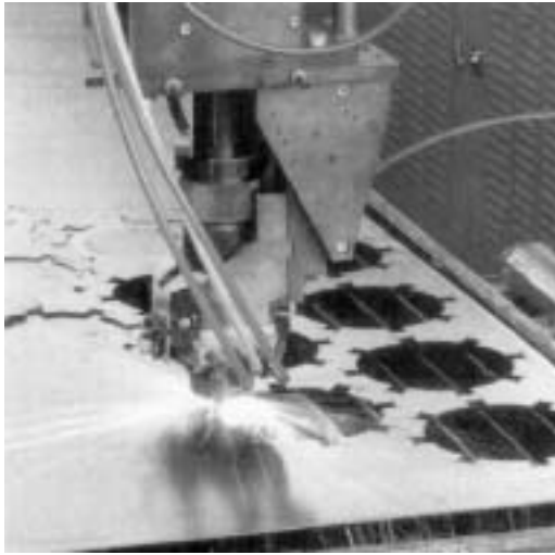
Fig. 21: Cutting various shapes by CO 2 laser
