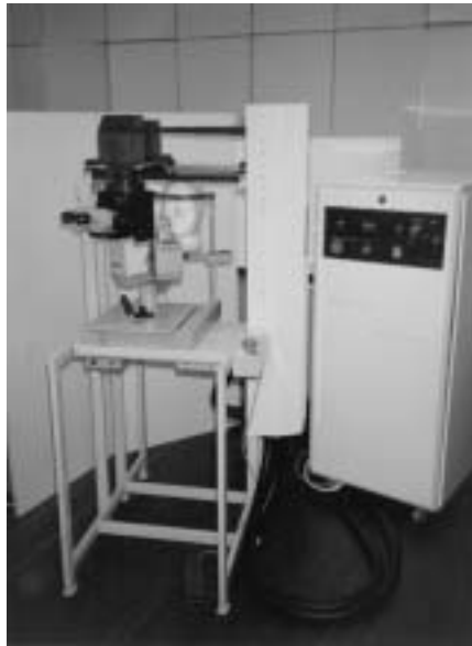
Fig.18: OFTLAS, a high-power pulse Nd:YAG laser, developed for eye microsurgery at FNSPE CTU
