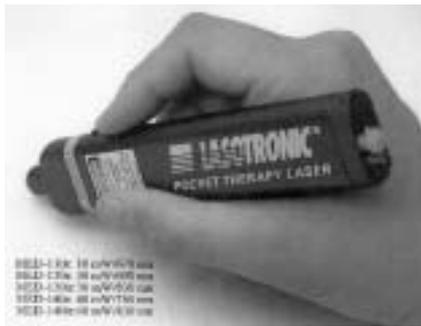
Fig. 19: Diode therapeutic laser by Lasotronic
