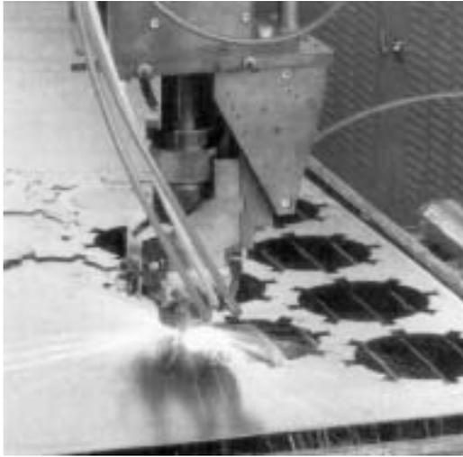
Fig. 21: Cutting various shapes by CO<sub>2</sub> laser
